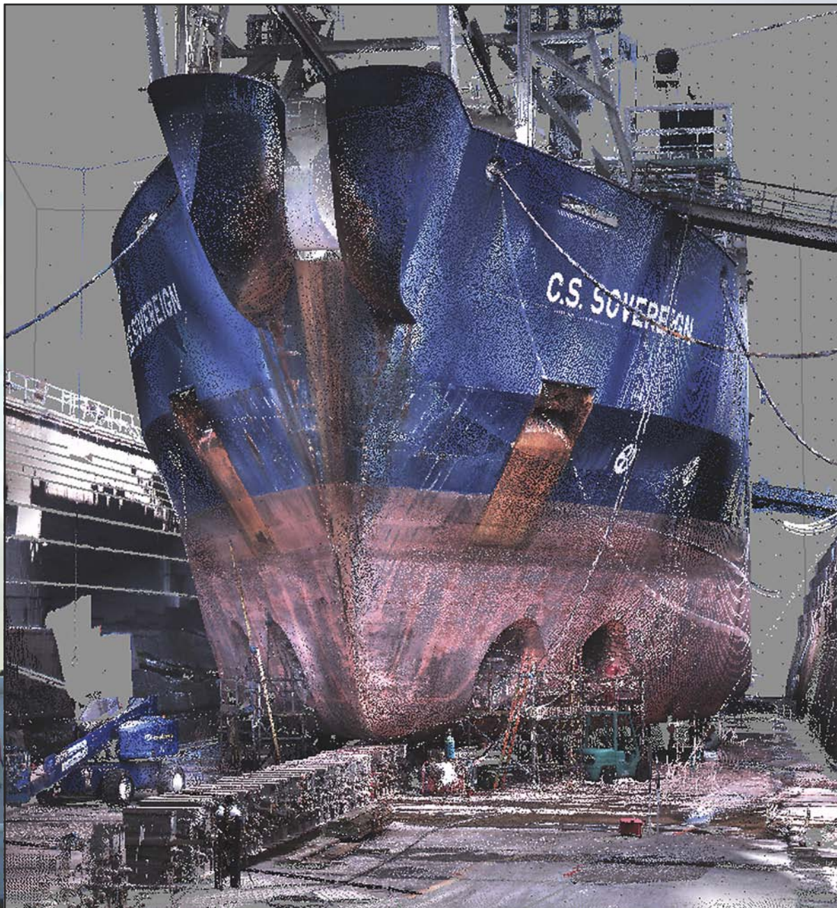
LEFT: This true-color 3D point cloud is of CSS Sovereign in dry dock.
